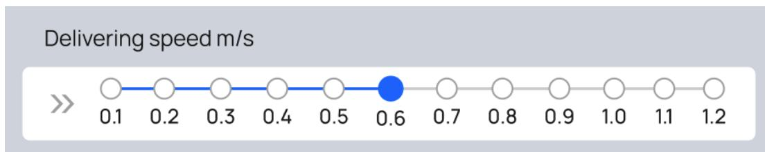
The robot can be configured to travel at a predetermined speed to a destination. The default speed is 0.8m/s, and this can be adjusted by dragging the cursor within the range of 0.1m/s(0.33ft/s) to 1.2m/s (3.93ft/s).
