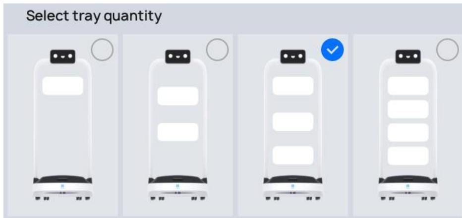
The number of trays can be selected according to the actual number of pallets actually assembled by the current robot. The selection range is 1 to 4. After modification, the number of trays in the robot schematic diagram on the left will be changed accordingly on the home page of each mode.
