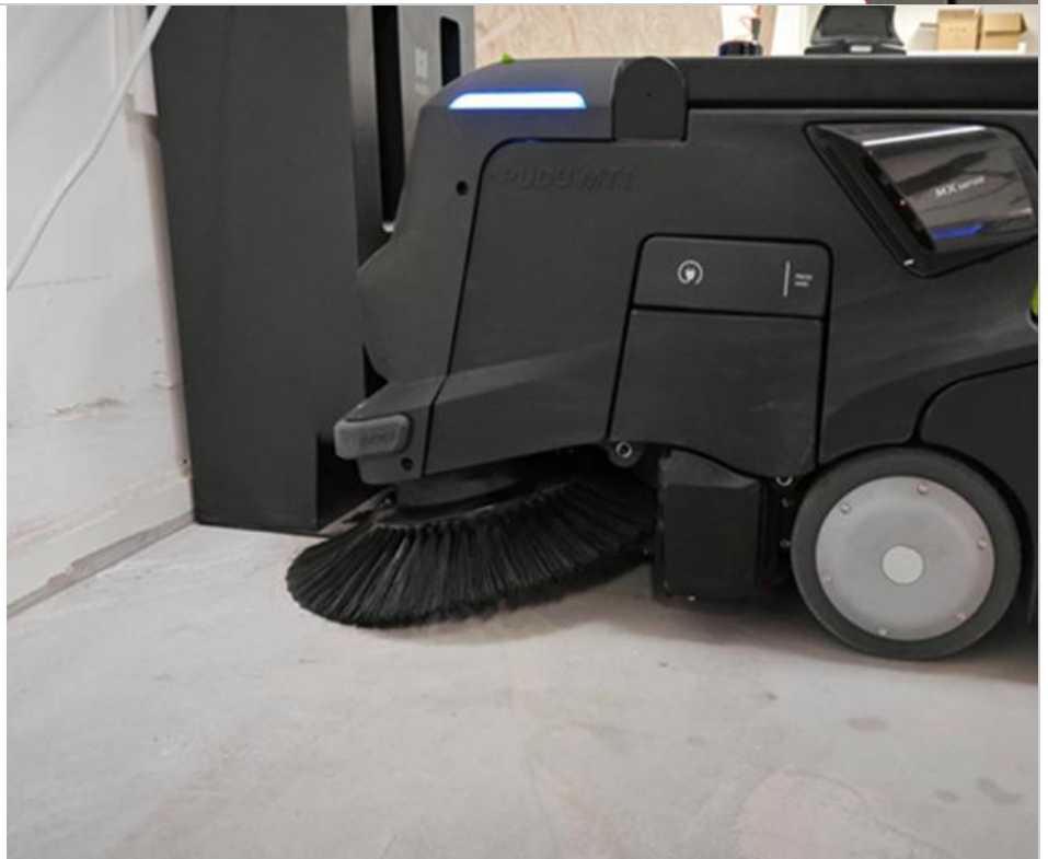
Robot docking with the charging station.
