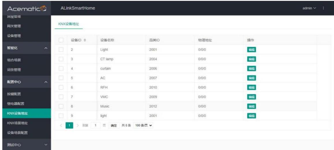
The screenshot shows the 'KNX设备地址' (KNX Device Address) configuration screen. The left sidebar has 'KNX设备地址' selected. The main table lists 9 devices:
