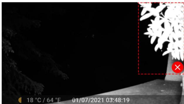
*Figure 9: Avoid close-up obstacles in front of the camera*
