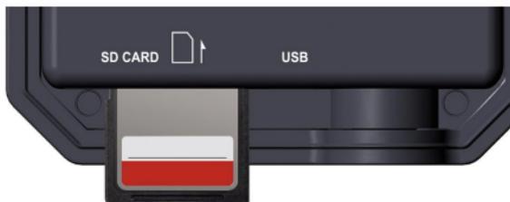
Figure 7: Inserting the SD Card
