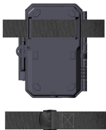
Figure 8: Mounting the Camera
