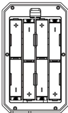
*Figure 6: Loading the Batteries*
