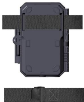
*Figure 17: Mounting the Camera*
