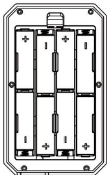
*Figure 6: Loading the Batteries*
