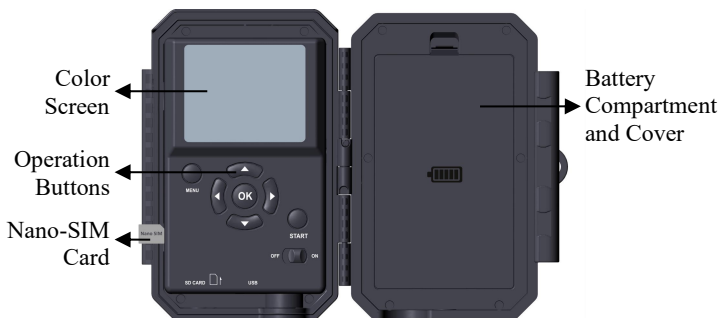
Figure 4: Inside View and Preinstalled SIM card
