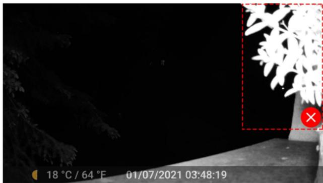
*Figure 18: Avoid close-up obstacles in front of the camera*
